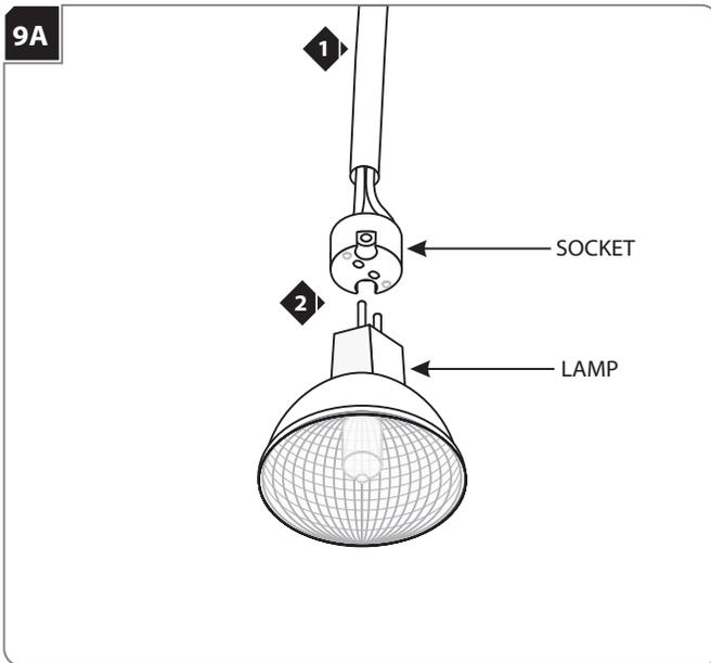
Use **MAX 75** Watt Type MR16 Halogen Lamp.
