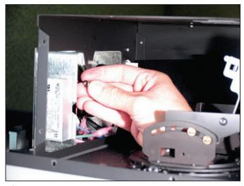
Remove the two thumb nuts inside the electrical box.
