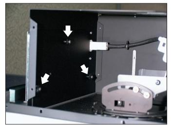
Remove the three thumb nuts on the access door.
