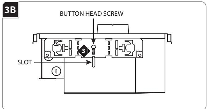
**NOTE:** Skip this section if installing the housing with adjustable bars.
