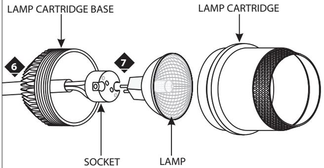
Use **MAX 50 Watt** Type MR16 Halogen Lamp.
