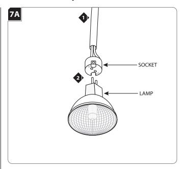
Use **MAX 75** Watt Type MR16 Halogen Lamp.
