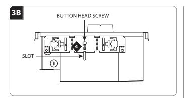
Place the button head screw through the square cut out of the butterfly bracket into the housing slot.
