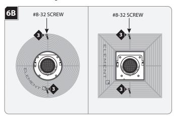
3 Secure the plaster ring in place with the two provided flat head #8-32 screws. Make sure that the screws penetrate through the drywall into the housing screw holes.
