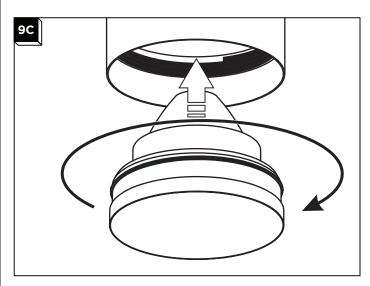
6 Install the reflector by inserting it into the bottom of the Cylinder and screw it in as far as it will go.
