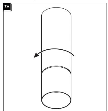
1 For the adjustable and wall wash fixture: the cylinder can rotate 358° to assist with aiming at the wall.
