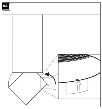
1 For the adjustable only: push up or pull down where the label is located to tilt the lower cylinder to the desired angle (o°-45°)
