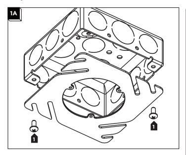
Prior to installing the drywall, attach the support plate to the junction box with the provided screws.
