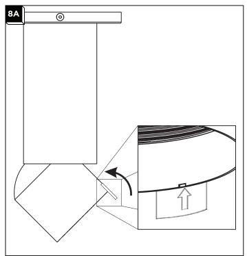
For the adjustable only: push up or pull down where the 1 label is located to tilt the lower cylinder to the desired angle (o°-45°).
