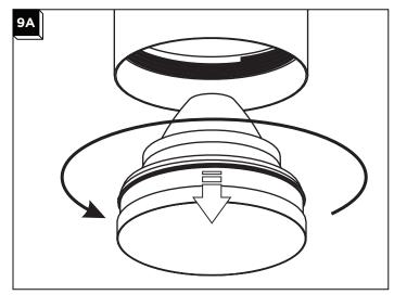
Remove the reflector by gripping the interior of the reflector and rotate counter-clockwise.
