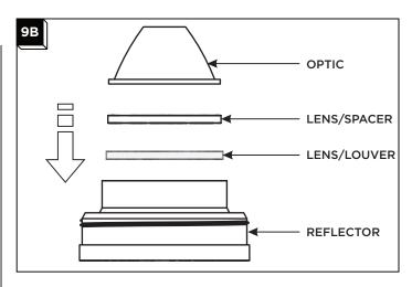
3 In the accessory reflector place the first lens or louver.
