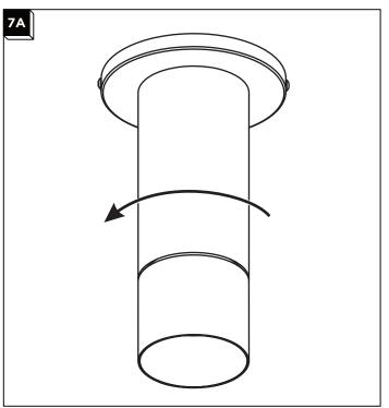
For adjustable and wall wash fixtures: the cylinder can rotate 358° to assist with aiming at the wall.
