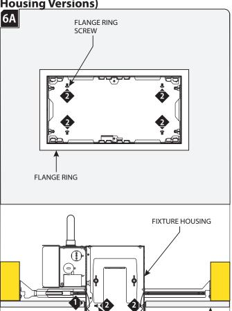
Insert the flange ring into the cut out and onto the fixture housing.
