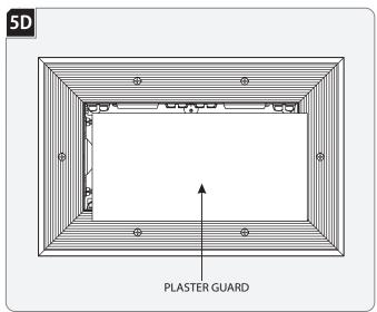
Install the plaster guard onto the housing with the provided double sided tape.
