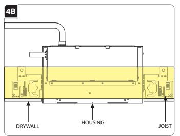
Align the cut out section of drywall with the housing and install drywall.
