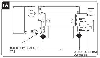
Rotate the tabs on the butterfly brackets 90° so that the adjustable bar openings are aligned.
