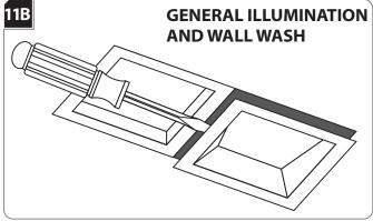
Remove the General Illumination and Wall Wash modules using a flathead screw driver to gently pry the module from the housing.
