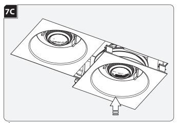
Align the spring clips on the module to the brackets inside the fixture housing and push the module completely in place.
