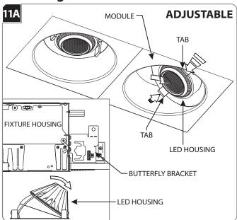
**WARNING:** Always squeeze the two tabs when adjusting the LED housing. Failure to do so will damage the finish.
