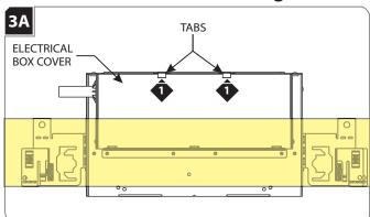
Push up on the tabs on the electrical box and remove the electrical box cover.
