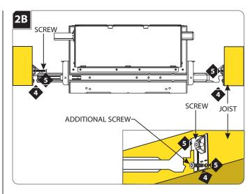
**NOTE:** The adjustable bars can be mounted to joists that are spaced 16" - 24" apart.
