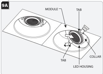
**WARNING:** Always squeeze the two tabs when adjusting the LED housing. Failure to do so will damage the finish.
