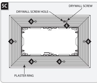
Secure the plaster ring to the ceiling using the provided drywall screw holes.
