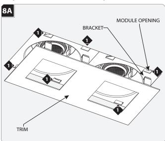
Align the brackets on the trim with the openings in the module(s).
