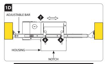
**NOTE:** The electrical box cover must be accessible for wiring the fixture. If the housing must be positioned so that the electrical box is not accessible, skip to section 3 to wire the fixture and revert back to this step to complete adjustments.
